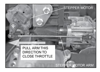
Figure 12. Throttle Positions 9/10 kW Units
